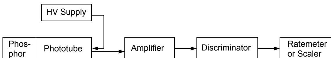
*Fig. 6.32. A Complete Scintillation Counter*
