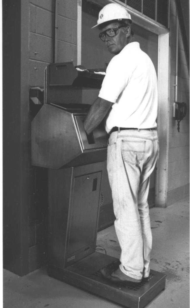
*Fig. 6.8. That's me at the Hand & Shoe Monitor*
