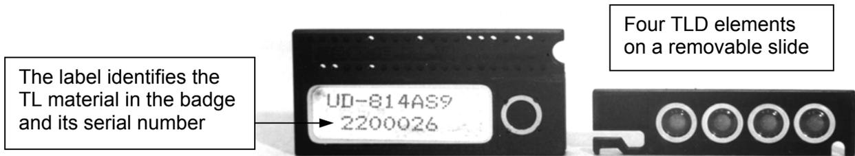
Fig. 6.46. TLD Holder: Rear View
