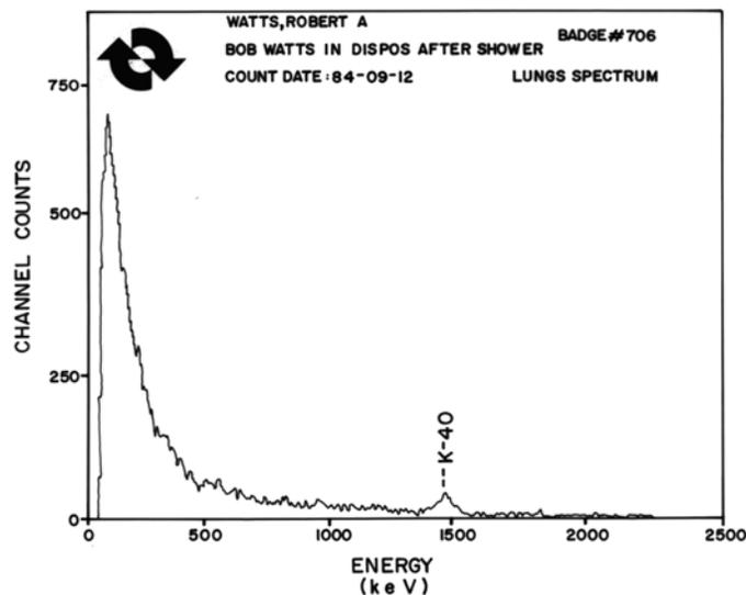
*Fig. 6.40. A typical Spectrum obtained with the Whole-Body Counter*
