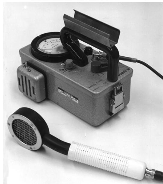
*Fig. 6.13. Portable Contamination Meter with Pancake Geiger Detector*
