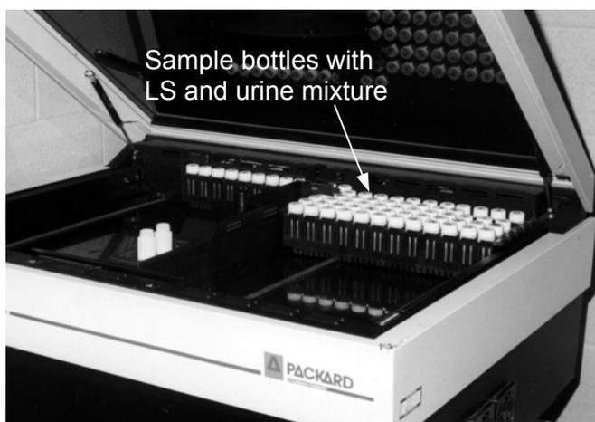
*Fig. 6.41. LSC for Bioassay Measurements*
