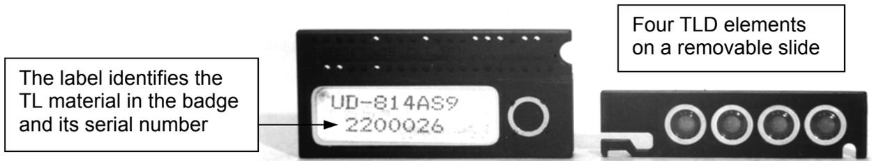
Fig. 6.46. TLD Holder: Rear View
