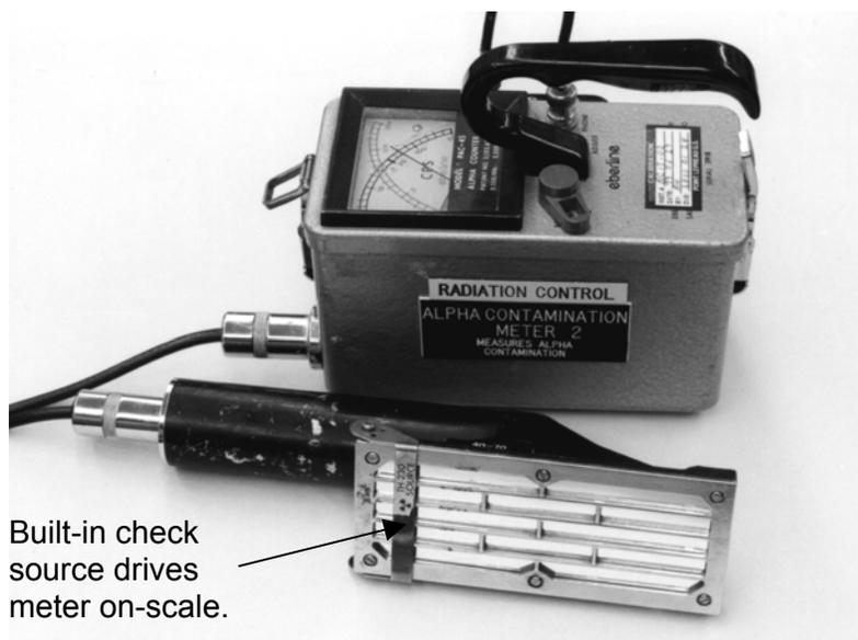
Built-in check source drives meter on-scale.
