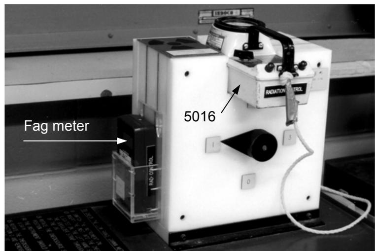
*Fig. 6.28. Instrument Check Source*
