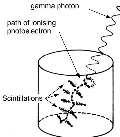
*Fig. 6.29. Gamma Absorption in the Phosphor*
