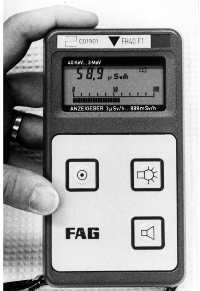
Fig. 6.21. The FAG Gamma Survey Meter with Analogue and Digital Displays
