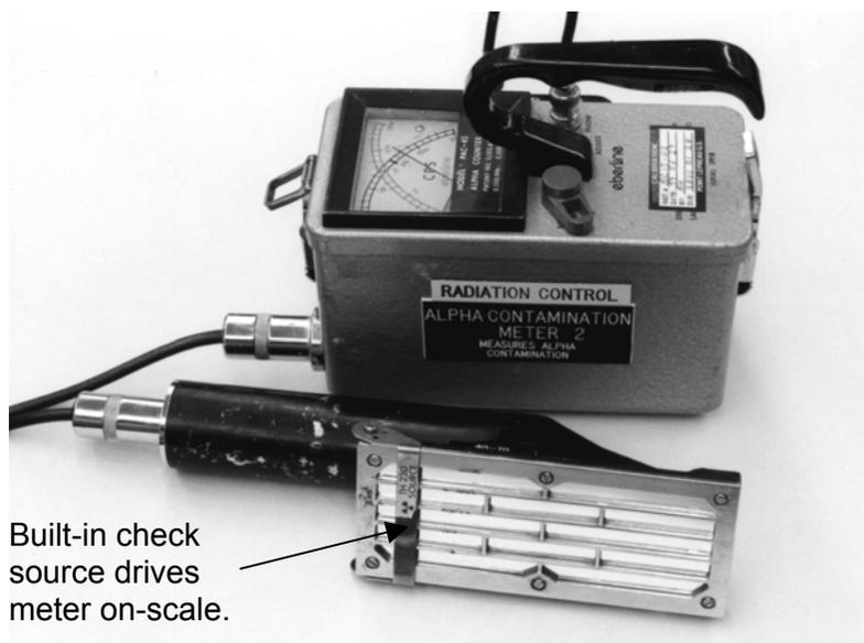
Built-in check source drives meter on-scale.
