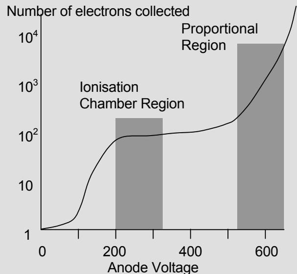
Fig. 6.7. Electron Collection versus Voltage
