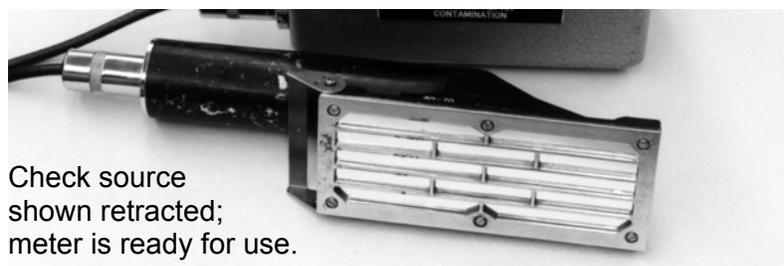
Check source shown retracted; meter is ready for use.
