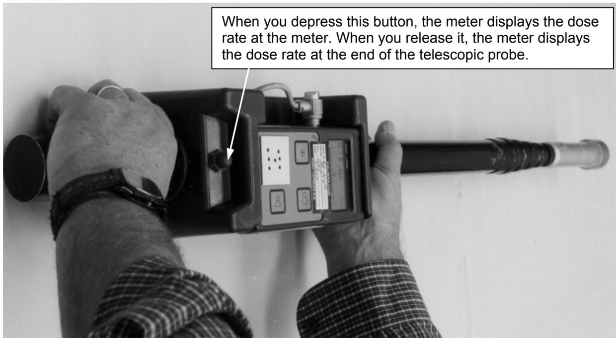
*Fig. 6.23. The Telescopic Unit Shown with its Extension*
