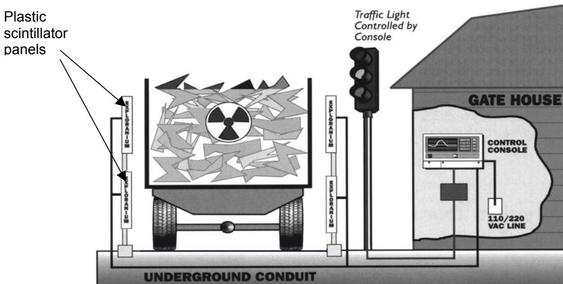
*Fig. 6.35. The Vehicle Monitor*
