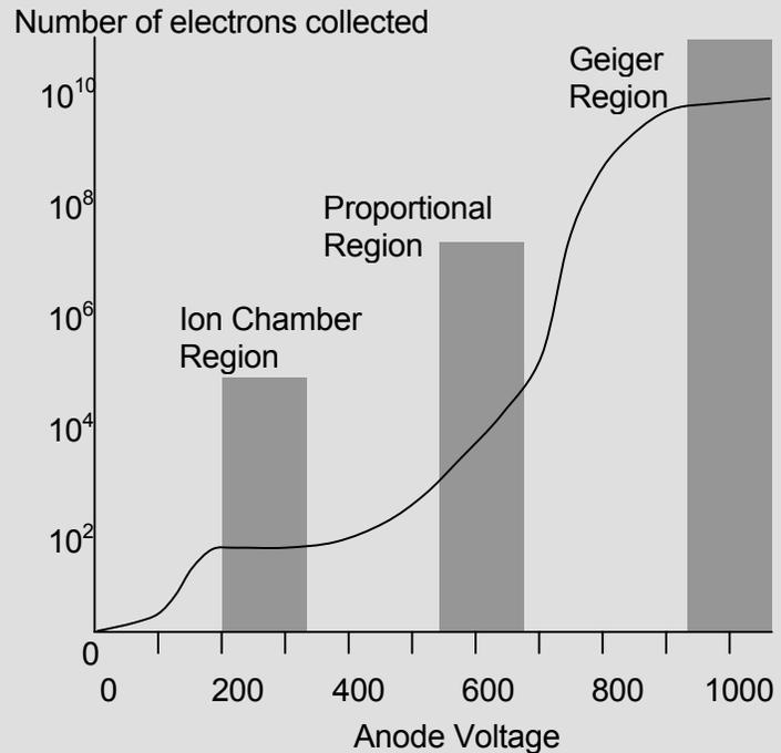
*Fig. 6.12. Gas-Filled Detector Characteristics*
